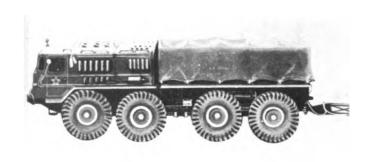
Figure 6-73. Heavy trucks. The 7.5-ton KrAZ-255B (above) is often used to carry bridge spans for the PMP folding bridge. The MAZ-535 (below) tows a launcher/trailer for surface-to-air missiles.
